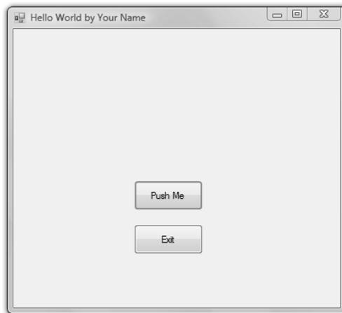
The Hello World form. The “Hello World” message will appear in a label when the user clicks on the Push Me button. The label does not appear until the button is pressed.
